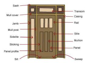
**Rails** – The rails are the horizontal crosspieces which hold the door panels in place. The centre rail is called the lock rail and is usually thicker than the other rails.
